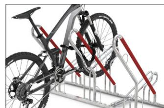
The striking detail of this free-standing bicycle parking system is the diagonal frame rest sheathed in signal red plastic. It protects every bicycle or e-bike against wanton or accidental wheel twisting and consequential damage to the rims. Integrated steel eyelets provide optimal theft protection. The spacing between hoops is generously laid out and ideal for bicycles with up to 55 mm wide tyres. Spacing is 500 mm or 540 mm
