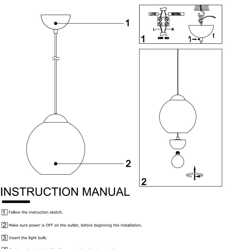
4 Go through point 1 to 2 before connecting the lamp to the power.
