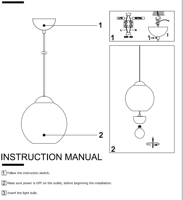
$\boxed{4}$  Go through point 1 to 2 before connecting the lamp to the power.
