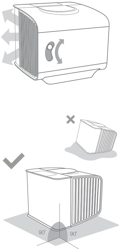
7. Move the trigger to adjust the airflow direction.
