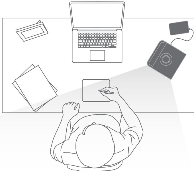
We have made sure that setting up your air cooler is quick and easy. evaLIGHT-plus is ready-to-use right after you unpack it. Following a few simple recommendations can help to ensure that your experience is as smooth as possible. The air cooler creates a personal comfort zone. To be in the center of that zone, place the device within 0.5 - 1.5 m (1.5 - 5 ft) of your position with its front grill facing you.
