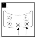
Briefly press cold/ambient dispense button to release internal water pressure from the machine. Remove the existing filter.
