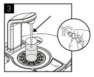
Turn on incoming water, allow service cartridge to fill. Dispense water using the cold button until the water appears pink. Briefly press the ambient button too. Repeat with sparkling button if present.
