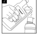
Add 25 ml of Bioguard Internal Sanitisation fluid to a clean and empty service filter cartridge and connect to the machine.
