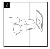
Plug in the power supply, cold, hot & sparkling tanks will automatically fill.
