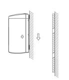
5. Push down slightly on the unit, then the unit and the mounting plate hook up tightly.
