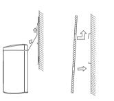
4. Hook up unit with right direction and press, make sure the unit is table by hooking up with the mounting plate.
