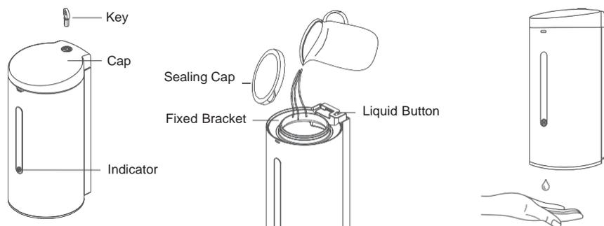
1. Insert the key into the lock to open the top cover after install the battery. Long press the setting button for about 3 seconds, then the LED light on with flashing 3 times
