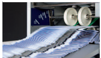
Large, extendable conveyor stacker for up to 300 folded sheets
