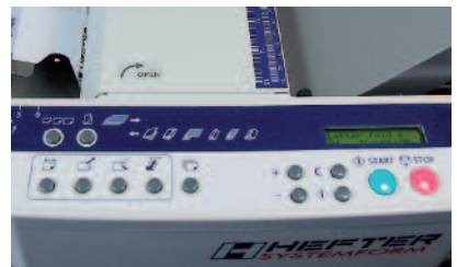
TF MEGA-A: Clear user panel with display, job and pre-counter
