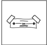
Attach the drill template to the wall with tape.
